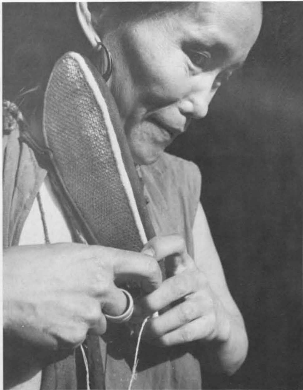
Shoemaker stitching on the sole, made of cloth layers tightly sewn together.
