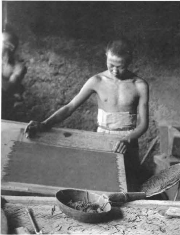
Incense-stick maker laying out the still moist sticks, made from ground wood of fruit trees put through a press.
